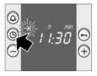
**5.** Press the  $\bigcirc$  clock button until the  $\rightarrow$ I end symbol flashes.
